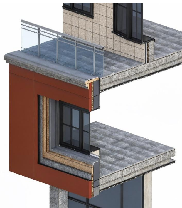
3D MATERIAL LAYER SECTION
